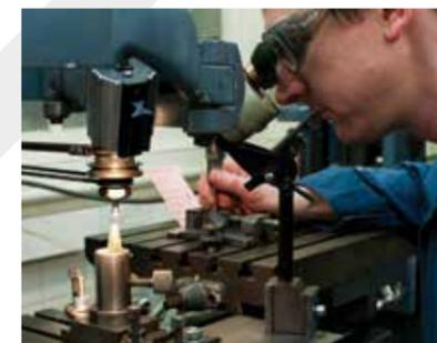
A master type set up on the pantograph machine Image: Julia Skupny
