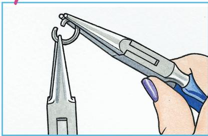
**1** Hold the jump ring with two pairs of pliers, either two flat-nosed or flat and round-nosed. To open, bring one of the pliers towards you.
