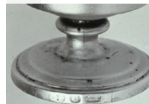
Solder lines either side of the mark.
