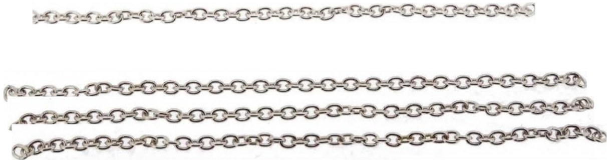
Figure 18: Manufactured chains of '925 Ag New' alloy, before (upper sample) and after accelerated lab tarnish test
