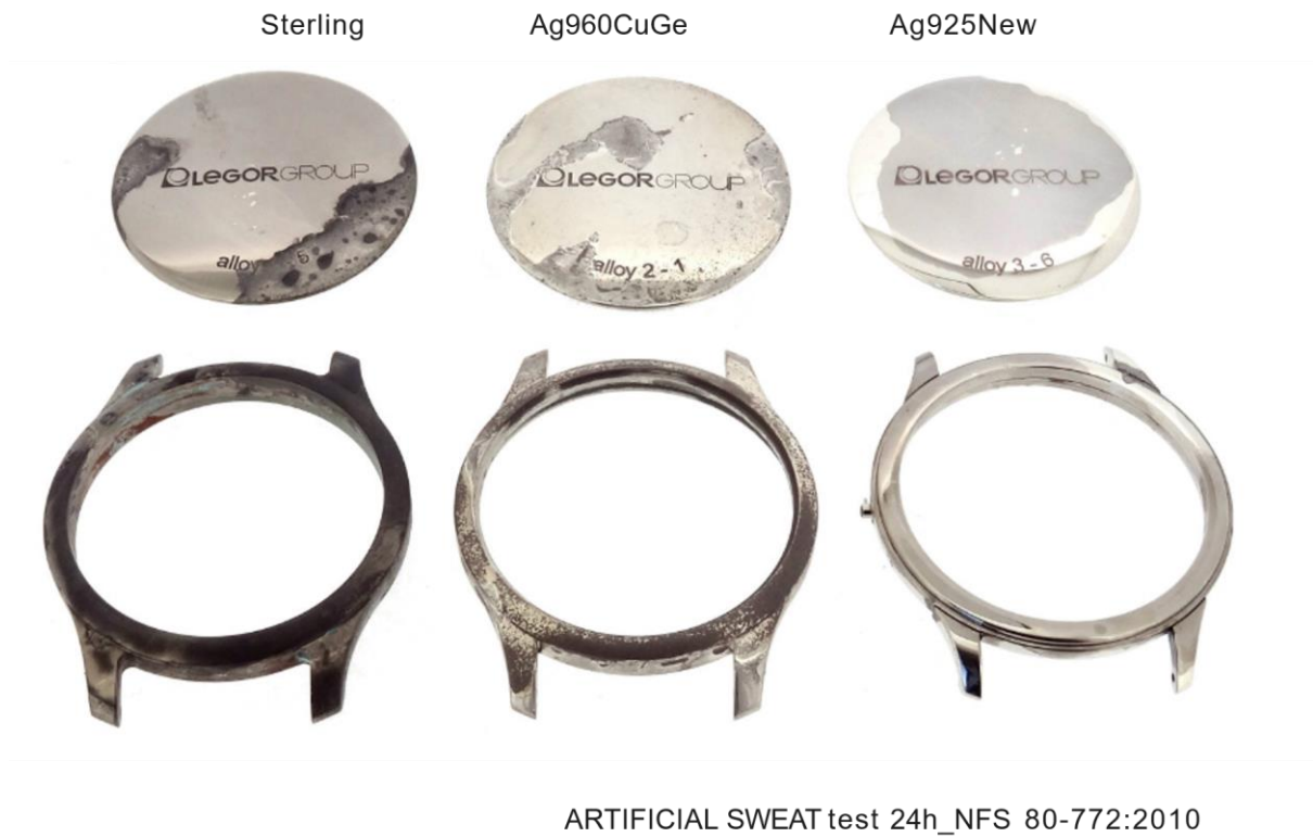
Figure 20: Manufactured watch cases of '925 Ag New' alloy compared to reference silver alloys after an accelerated lab tarnish test
