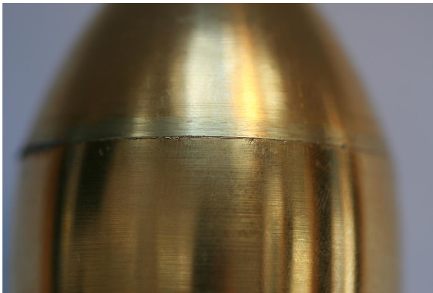
Figure 3, 1/3 trial spinnings, even thickness and accurate seam alignment.
