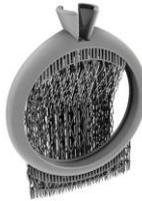
*Figure 19 Feeders and supports for solitaire model 5*
