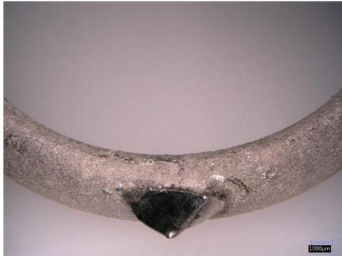
*Figure 27 Feeder residual on a ring's surface*
