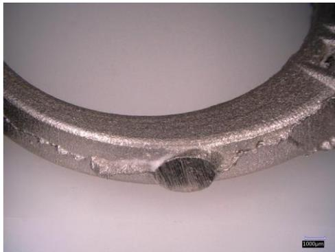
*Figure 37* Material excess on the side of the cast ring (fin defect)
