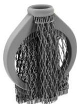
*Figure 21 Feeders and supports for solitary model 8*
