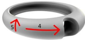
**Figure 32** Roughness measurement direction for cast solitaires and trilogies
