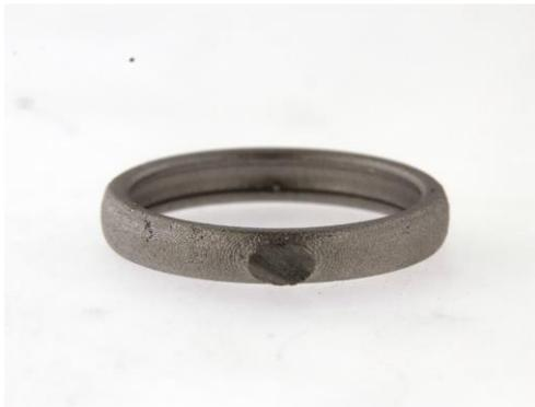
**Figure 32** Cast band model 4 after sandblasting
