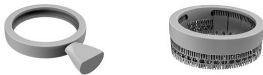
*Figure 16 Feeders and supports used for the production of band model 1*
