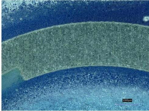
**Figure 88** “As-print” SLM™ band after etching, 50X
