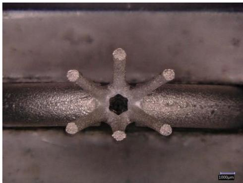
**Figure 47** Deformation of the prongs in cast solitaire model 4
