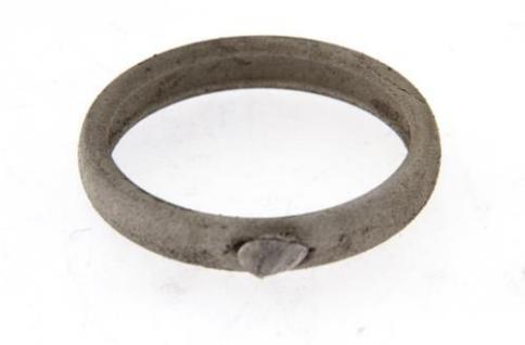
**Figure 30** Rough band model 4 produced using casting
