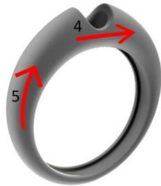
**Figure 31** Roughness measurement directions for SLM™ solitaires and trilogies
