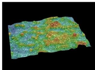
*Figure 34 Surface roughness of a rough SLM™ band , 300X*
