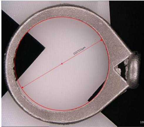
**Figure 46** Cast solitaire model 8 with evident ovalization
