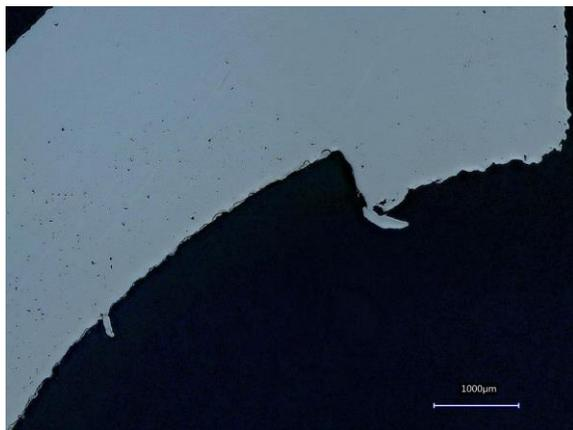
*Figure 77 Inter-hatch porosity in a section of an SLM™ ring*
