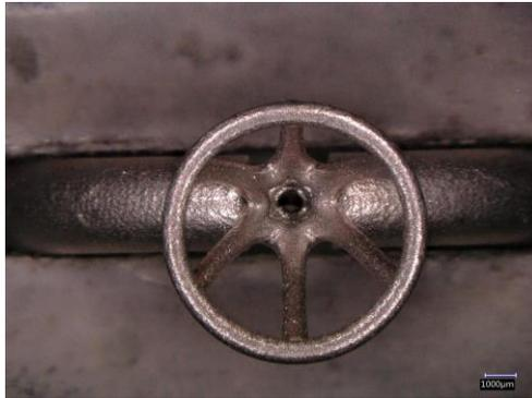
**Figure 48** Added ring to stabilize the position of the prongs in the cast solitaire model 4
