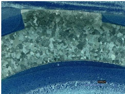
*Figure 78 As-cast band after etching, 50X*
