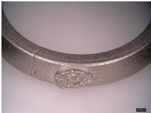
**Figure 49** Cracked ring shank
