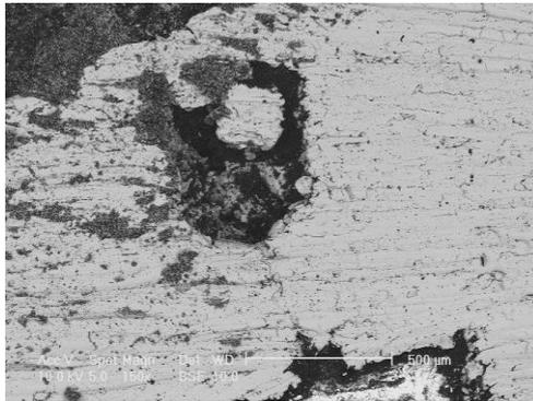
*Figure 51 Extension of the cavity on the other half of the sectioned ring shank*
