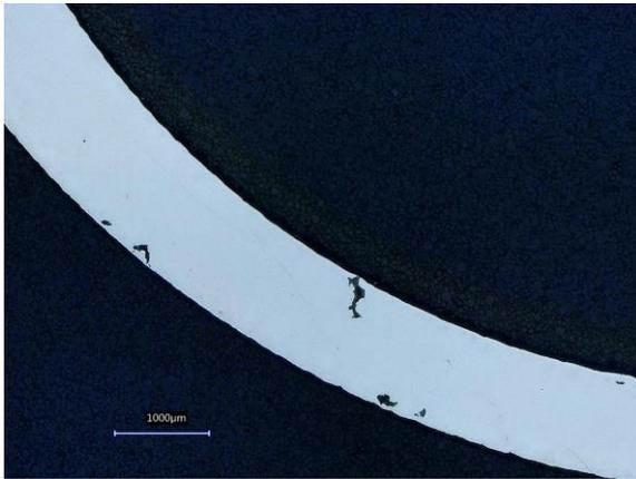
*Figure 74 Cavity in a section of a cast ring*
