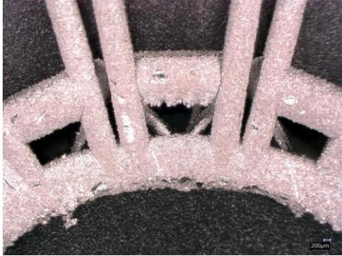
**Figure 29** Internal supports of trilogly model 2
