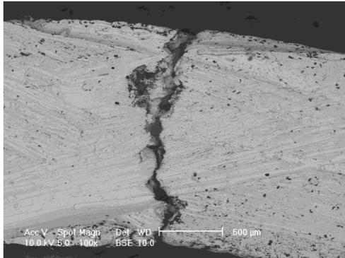
*Figure 50 Internal cavity in a cast ring shank, corresponding to the fractured section.*
