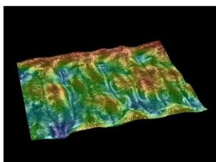
*Figure 35 Surface roughness along a horizontal wall of a rough SLM™ band, 300X. The parallel traces left by the laser scans are visible.*
