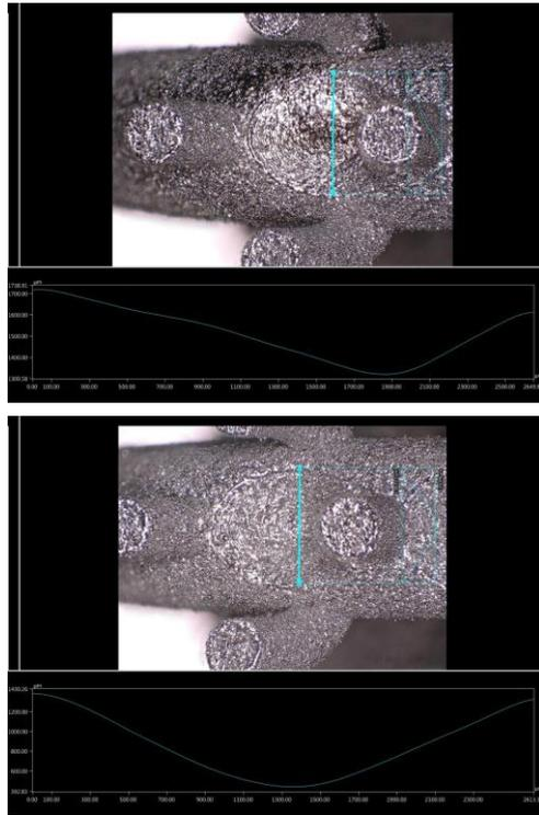
*Figure 53 Defect on a trilogly ring surface (upper image) compared to the surface of a standard one (lower image)*
