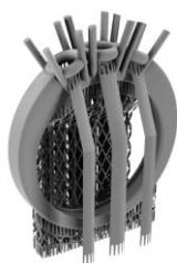
*Figure 24 Feeders and supports for trilogy model 1*
