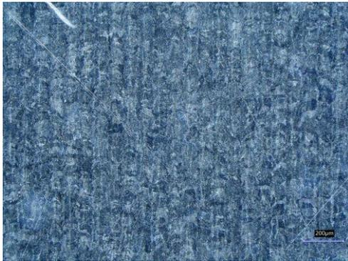
**Figure 89** “As-print” SLM™ sample, 200X
