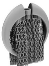
*Figure 23 Feeders and supports for solitary model 16*
