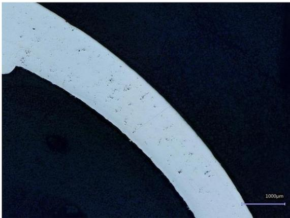
*Figure 75 Shrinkage porosity in a section of a cast ring*
