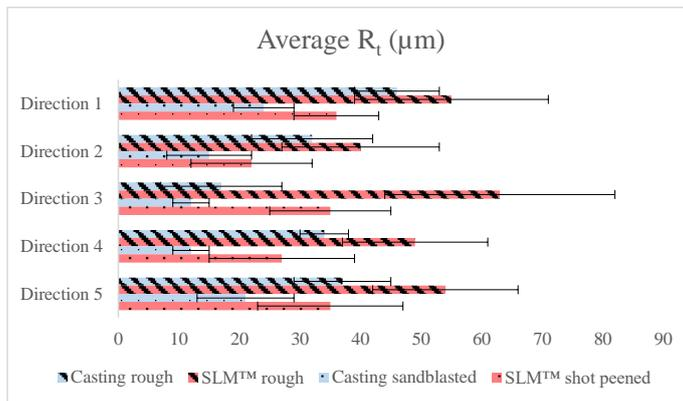
**Figure 33** Average roughness for SLM<sup>TM</sup> and cast pieces
