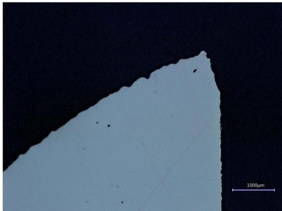
*Figure 76 Gas porosity in a section of an SLM™ ring*
