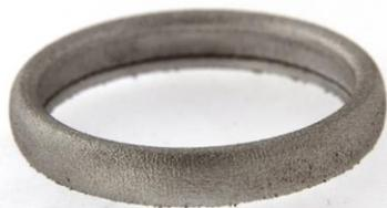
**Figure 33** SLM™-produced band model 14 after shot peening
