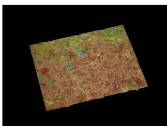
*Figure 36 Surface-roughness along a horizontal wall of rough cast band, 300X*
