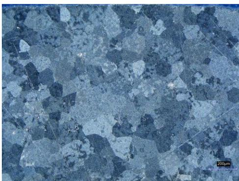
*Figure 79 As-cast sample, 200X*
