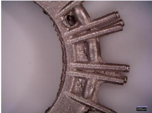
**Figure 38** Example of finning caused by investment rupture
