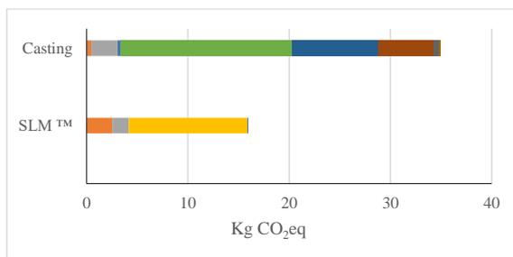
**Figure 105** Kilograms of equivalent CO<sub>2</sub> produced through each technique
