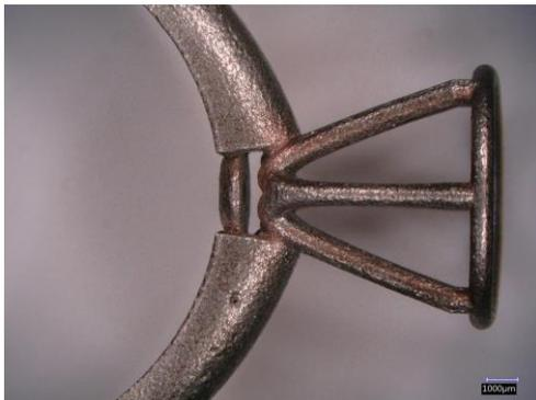
**Figure 39** Emerging cavity on the surface of a solitaire model 4, probably caused by an investment detachment that was trapped in the molten metal
