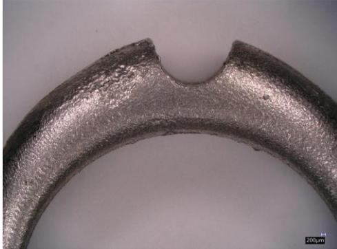
*Figure 42 Irregular surface on cast solitaire model 7*
