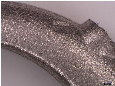
*Figure 41 Depressions probably caused by detached fragments of investment floating on the surface of the molten metal*
