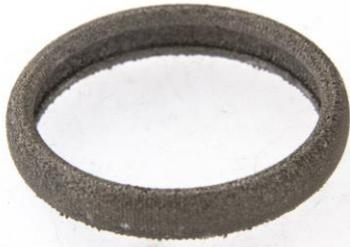
**Figure 31** Rough band model 4 produced using SLM™
