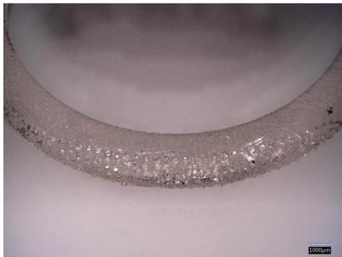
*Figure 26 SLM<sup>TM</sup> support residuals on a ring's surface*
