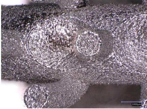
*Figure 52 Surface swelling of an SLM™ trilogly model*
