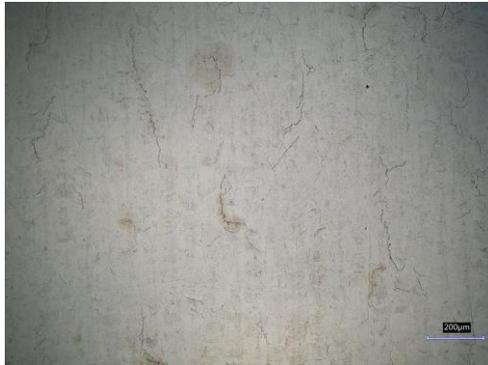
**Figure 80** Micro-cracks observed in the SLM™ band after etching
