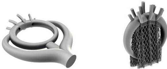
*Figure 25 Feeders and supports for trilogium model 2*
