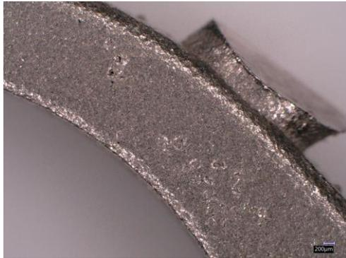
**Figure 44** Surface porosity on cast solitaire model 8
