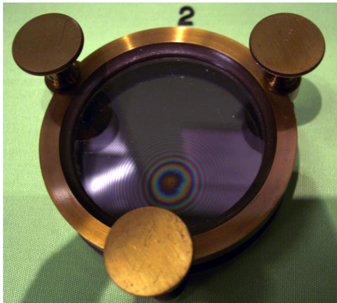
Figure 8: Apparatus formerly on display in the Science Museum showing Newton's rings.
