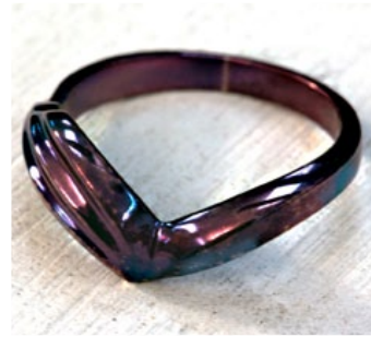
When using higher melting point solders, palladium will take on a surface oxidation that is blue-violet.
