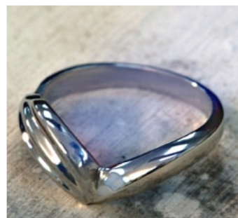
When using higher melting point solders, palladium will take on a surface oxidation that is blue-violet.
