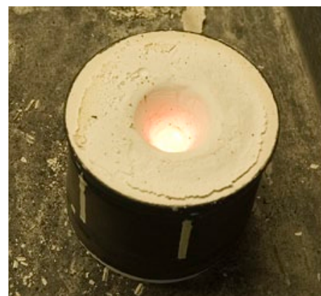
Just-cast palladium flask at Unique Settings, New York, NY, USA
